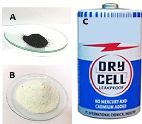
Fig. 1 The materials used in this study are (A) graphite powder from the battery waste, (B) commercial detergent, and (C) a ZnC battery.
