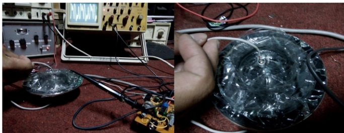
Fig. 4 A test to determine the frequency of the solution (A) by submerging a mic condenser into the solution (B).
